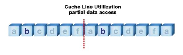
**Image caption:** Although the cache in principle is filled optimally, the majority of the data contained in it remains unused.
