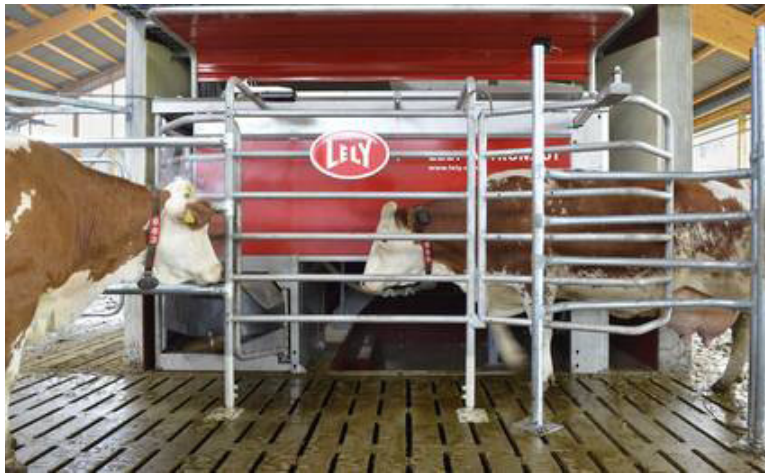
Lely's milking system collects data per cow on milk production and cow health. This alerts the farmer on time to any changes, allowing him to devote his attention to the cows that need it most.
