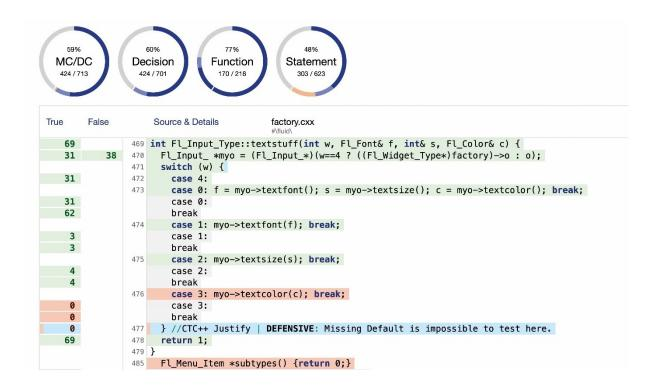
The screenshot of the Code Coverage Analyzer Testwell CTC++ shows the tested code parts in green and untested code in red. The code in line 477 is also untested (recognizable by the red marking on the left) - however, a justification has been inserted for this, which states that this line of code is not testable. This "justified" part of the code is then displayed in blue.
